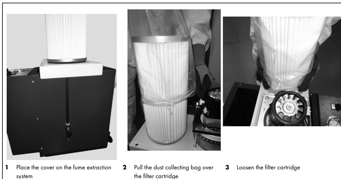
Fig. 5 Changing the filter
