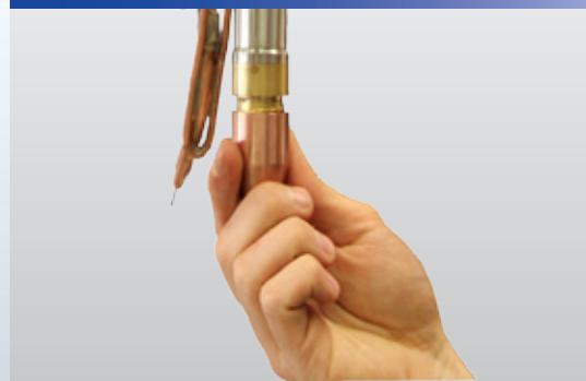
Step 4: Screw on the gas nozzle. Finished!
